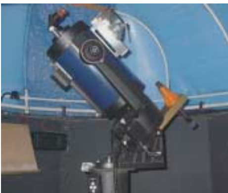
My Meade LX-10 with the Tuthill Polar alignment scope installed—just waiting for a clear night.
